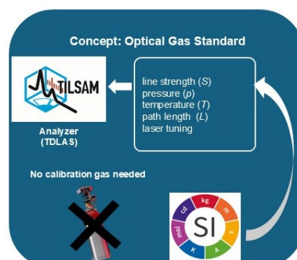
Fig 1: Sketch of an optical gas standard. The analyzer operates according to the TILSAM method.
